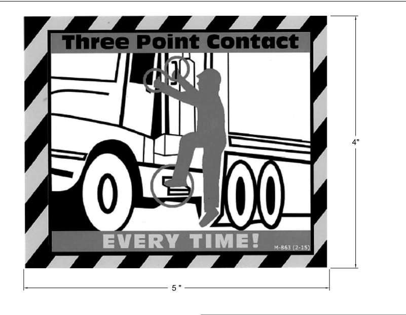
THERE SHALL BE A PERMANENT DECAL AFFIXED ON EACH DOOR. THE SAME PERMANENT DECAL SHALL BE AFFIXED BY EACH BODY LADDER. MEASUREMENTS OF DECAL ARE REFERENCED ABOVE.
